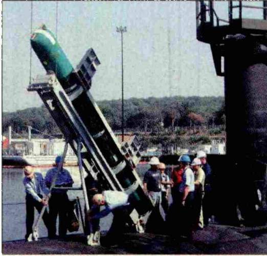
Boeing unmanned underwater vehicle: could locate underwater mines, spy, attack other vessels
